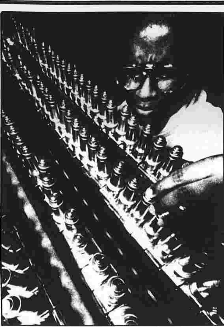
Big wheel Harvey Barbee of Invacare Corp. inspects a rack of castor forks used to support the front wheels of the "Jaguar" and "Rabbit" model wheelchairs, designed specifically for children. They are made at the company's plant in Elyria, Ohio.
